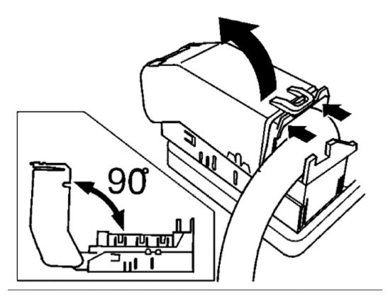
Disconnect the connector from the control module Press the catch and pull up the connector. Pull the connector up a maximum of 90 degrees (any more and the connector will break).
