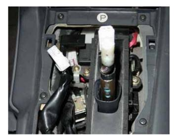
9. Gently pull out the center trim and gain access to the Climate Control unit and the Radio.
