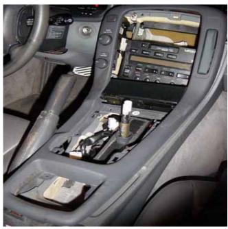
10. Remove the harness that attached to the center trim.
