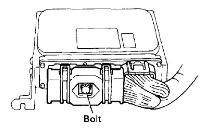
Fully loosen the bolt and disconnect the 2 ECM connectors, and remove the ECM.
