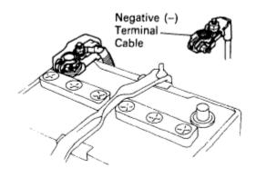
1. DISCONNECT NEGATIVE (-) TERMINAL CABLE FROM BATTERY. CAUTION: Work must be started after 90 seconds from the time the ignition switch is turned to the LOCK position and the negative (-) terminal cable is disconnected from the battery.
