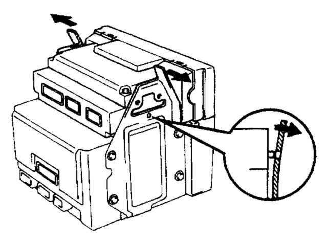
Open the brackets on the outside, release the connection of the claws and remove the air conditioner control assembly
