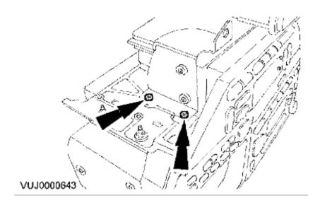
Remove the control assembly screws
