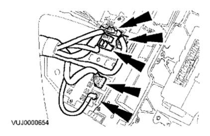
Remove the center control panel. Disconnect the audio system electrical connector.
