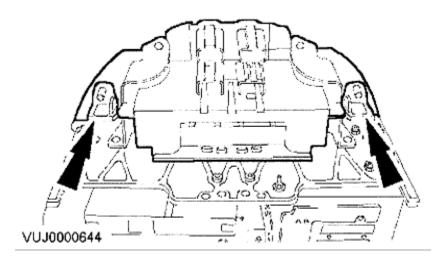
Remove the control assembly
