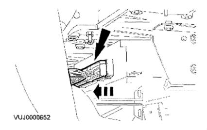
Disconnect the climate control unit electrical connectors
