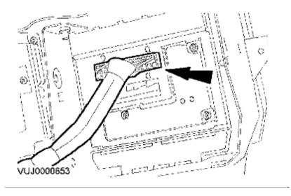
Disconnect the satellite navigation screen electrical connectors ,lf applicable
