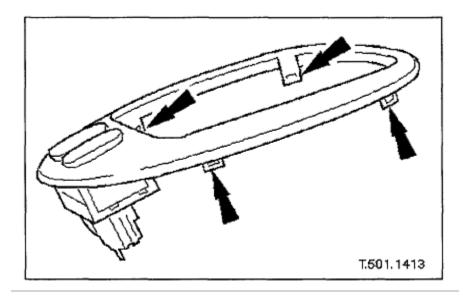
3. Using a thin plastic lever and exercising care to avoid damaging veneer surface, release the four surround tangs from the 'J' gate.
