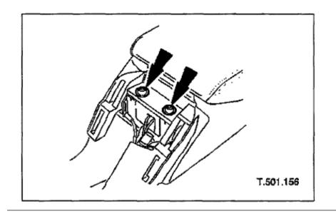
Remove console and trim cover and slacken and remove the two rear securing bolts
