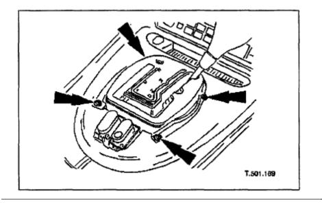
4. Slacken and remove the four center console veneer panel securing screws and remove the mounting plates.
