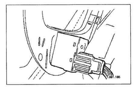
Disconnect multiplugs from Sport mode and Cruise Control on/off switches.
