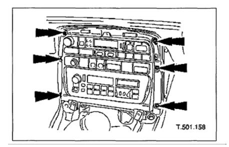
Remove radio console securing screws and position console for access
