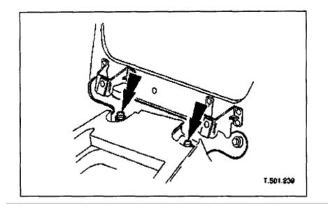
7. Slacken and remove the two forward securing bolts.
