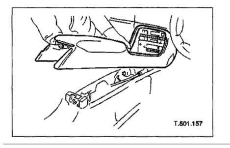
8. Position console for access, disconnect cigar lighter and valet switch harness multiplugs, lift console clear of 'J' gate and remove from vehicle.
