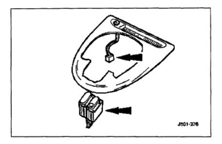
Position the veneer panel for access and disconnect the panel switch multiplugs
