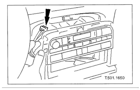
Disconnect air conditioning control module harness multiplug and cut and remove securing tiestrap
