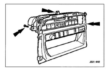
6. Remove remaining switch control module central securing screw and withdraw module from vehicle.
