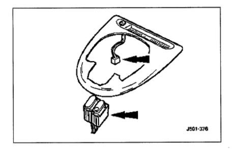
5. Noting orientation of switches, depress tangs and remove switches from surround.
