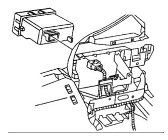
1. Connect the electrical connectors to the HVAC control assembly.
