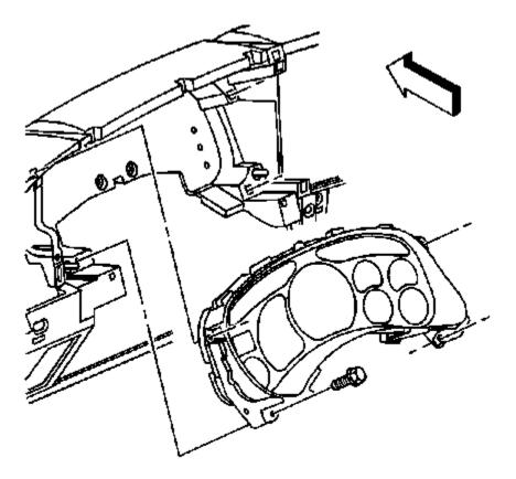
Remove the screws that retain the IPC to the instrument panel (I/P) assembly
