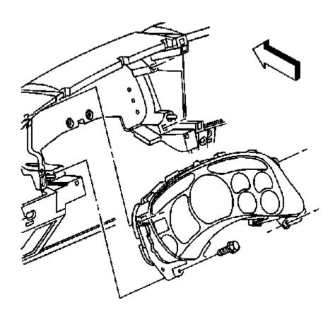
Remove the screws that retain the IPC to the instrument panel (I/P) assembly www.autoecu.com
