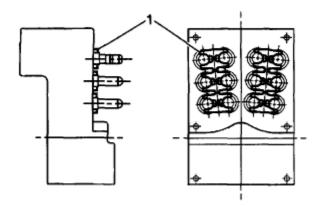
2. Install two wave springs (1) between the EBTCM and BPMV. Use locations and orientation noted during removal. Notice: Refer to Fastener Notice in Service Precautions.
