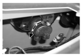
4. Pull the flat connector attached to the white wire from the headlamp bulb shield.
