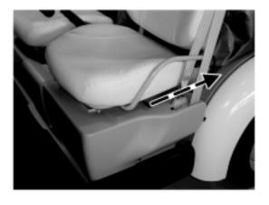
the rear and slide the seat to the desired position. Release the lever to lock the seat in the new position.
