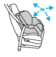
8. Check from time to time to be sure that there is no slack in the lap/shoulder belt. The shoulder belt must be snug to keep the lap belt tight during a collision.
