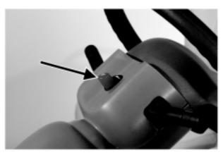
mode selector switch in all positions. The hazard flasher switch is located on top of the steering column, right behind the steering wheel. Depress the switch to activate the hazard lights. To turn off the hazard lights, depress the switch again.
