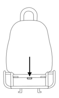
4. Clip the tether strap to the anchor as shown.
