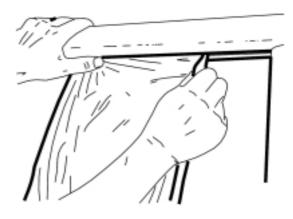
5. Wrap and fasten the large upper attaching strap around the B-pillar.
