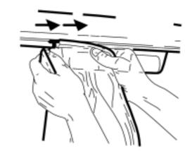
5. Unfasten the three side weather enclosure mounting hooks from the openings in the frame rail.
