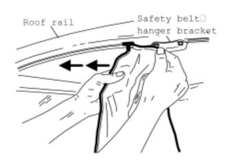
3. On four-passenger vehicles, insert the side weather enclosure rear hanger ("T" section) into the slot on the underside of the roof rail behind the safe
