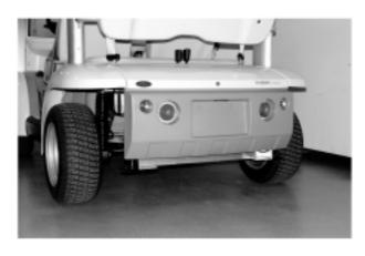
outboard lamps are the rear turn signal lamps.
