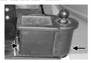
2. Remove the five screws from the bottom of the cover. Remove the cover.
