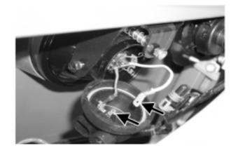
3. Install and rotate the headlamp bulb shield clockwise.
