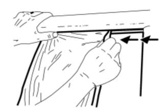
9. On four-passenger vehicles, remove the side weather enclosure rear hanger ("T" section) from the slot on the underside roof rail by the safety belt hanger bracket.
