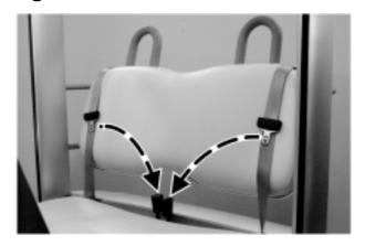
The front passenger and rear seat (if equipped) have cinch tongues to help install a child safety seat tightly.
