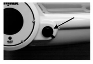
a rubber plug protecting the power point. To use the power point, remove the rubber plug and insert the desired accessory plug. Always keep the rubber plug inserted into the power point when not in use.
