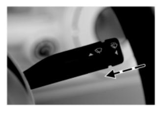
Release the lever to stop the washer and turn the wiper off.
