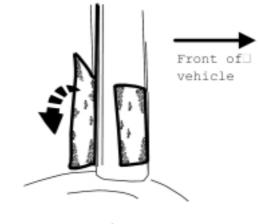
7. Pull apart the two 1-inch attaching straps.
