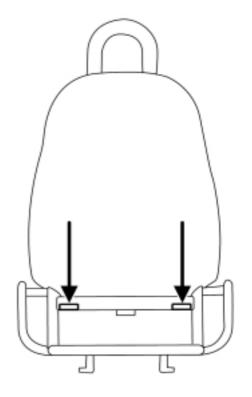
Follow the child seat manufacturer's instructions to properly install a child seat with LATCH attachments. Two plastic LATCH guides can be obtained at no charge from any TH!NK dealer. They snap onto the LATCH lower anchors in the seat to help attach a child seat with rigid attachments. The guides hold the seat trim away to expose the anchor and make it easier to attach some child seats.
