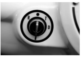
system. It also functions as a gear selector by placing the drive mode selector switch key in one of four modes: R (Reverse), (OFF), T (Turf), and D (Drive).
