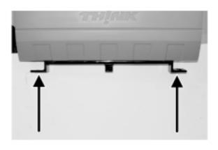
Additionally, when shipping or transporting, all four tow/tie down hooks *must* be used to prevent damage.
