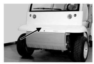
2. Observe the level of fluid in the reservoir on the right side of the compartment.
