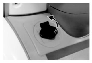
5. Align the GFCI charger cord with the charge inlet and fully insert the plug into the outlet.
