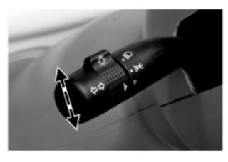
arrow indicator will flash on the instrument cluster indicating that the turn signal is on.
