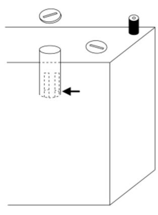
bottom of the slotted cup. Do not overfill.
