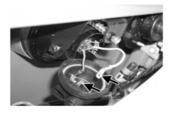
5. Push and squeeze the two bulb retainer wires to disengage them from the headlamp housing. Remove the headlamp bulb.
