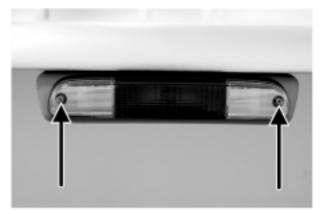
2. Rotate the bulb socket counterclockwise and pull out to access the bulb.
