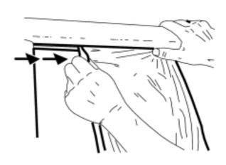
4. Remove the rear weather enclosure hangers from the slots behind the high-mount stop lamp.
