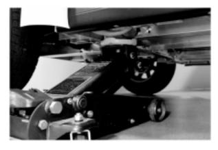
• The proper jack lifting points are not utilized.
