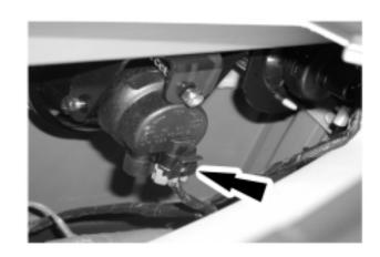
3. Rotate the headlamp bulb shield counterclockwise and flip down to access the bulb connectors.
