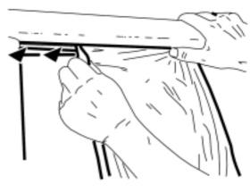
11. Zip the two rear weather enclosure to side weather enclosure zippers.
