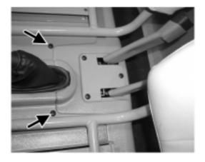
3. From both sides of the vehicle, remove the two push pins. (Driver side shown; passenger side similar)
