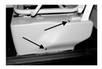
4. From both sides of the vehicle, remove four bolts from beside the seat frame. (Driver side shown; passenger side is similar.)
