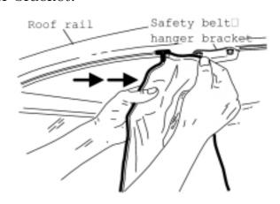
11. Remove the side weather enclosure front hanger from the slot on the underside of the roof rail in front of the safety belt hanger bracket.
