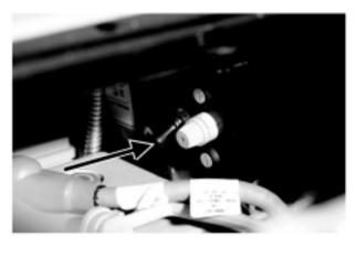
located below and behind the parking brake lever within the seat stanchion (battery cover). It is a black rubber switch and faces the front of the the vehicle. It is not encouraged to blindly reach down through the driver's side opening on top of the seat stanchion cover when the cushion is removed.
