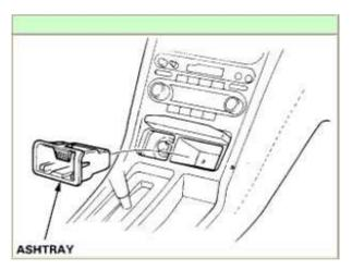
Take out the ashtray and remove the two screws from under the ashtray
