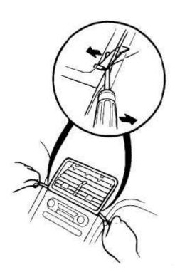
2. Remove the two screws behind the clock, then remove the center air vent.
