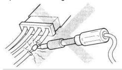
Be sure to install the harness wires so that they are not pinched or interfering with other parts.
