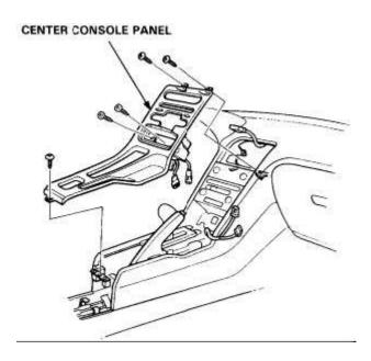
5. Remove the three screws and center console panel, then disconnect the 3P connector and 4P connector from the floor wire harness.
