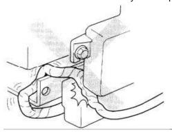
Make sure all SRS ground locations are clean and grounds are securely fastened for optimum metal-to-metal contact. Poor grounding can cause intermittent problems that are difficult to diagnose.
