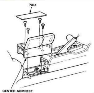
Remove the four screws, then remove the center armrest
